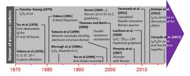
Raman spectroscopy applied to the study of carbons containing aromatic clusters started in the early 1970's and has been improved since then, but still some questions remain unsolved. In  $^1$  and  $^2$  we present its state of the art.
