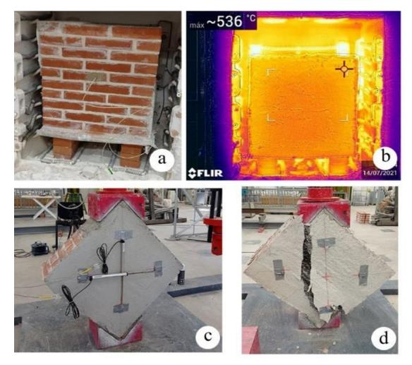
Experimental campaign. (a) Masonry wall. (b) High temperature inside oven (c) Shear tests on a TRM retrofitted masonry wall (d) Damaged wall
