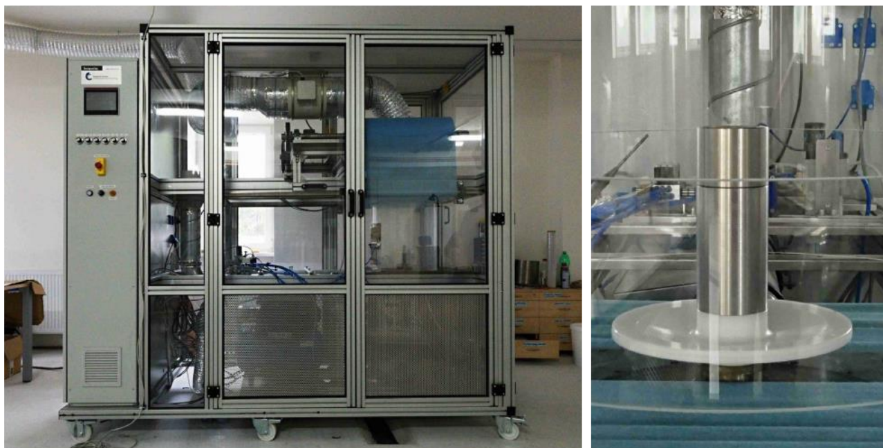
Demonstrator NANOCENT (left) and fiber-forming rotating hollow disk (right)
